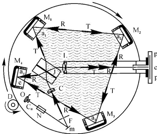
Fig 1. Design of the Sagnac setup
