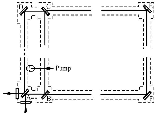
Fig 2. Light channels in the Michelson-Gale experiment. AF = 620m, AD = 340m.
