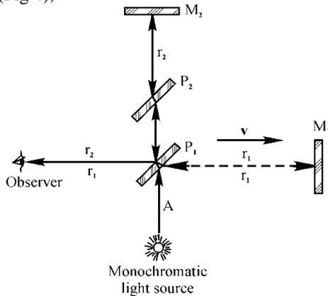
Fig 4. Scheme of the Michelson interferometer.
