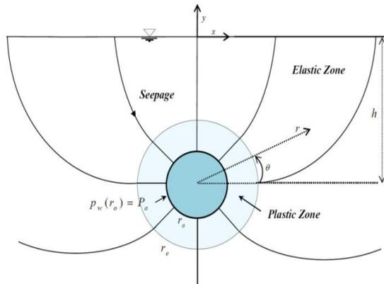
**Fig.1** Seepage pattern in underwater tunnel
