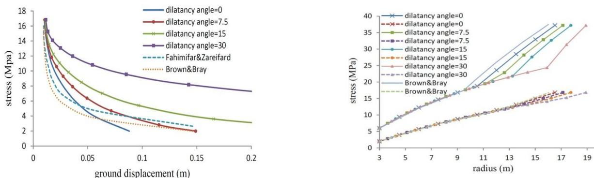
**Fig.2 a.** Ground response curve, **b.** Radial and tangential stresses at the plastic zone (plain lines denote tangential stress while dotted lines represent radial stress),  $h=300$  m
