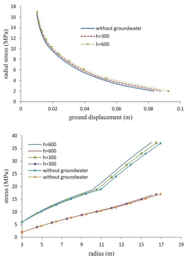
**Fig.3 a.** Ground response curves, **b.** Radial and tangential stresses at plastic zone (Plain lines denote tangential stress while dotted lines represent radial stress),  $\phi = cte$
