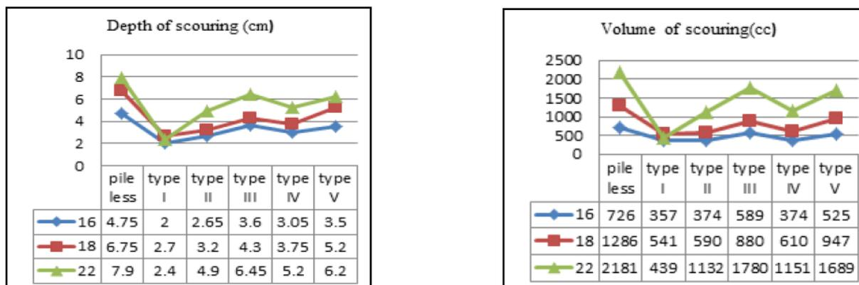
Figure.8 The diagram of maximum scour depth and volume given different types of pile positioning (Source: author)
