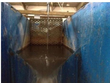
**Figure.1** The triangular weir to measure the flow rate (Source: author)
