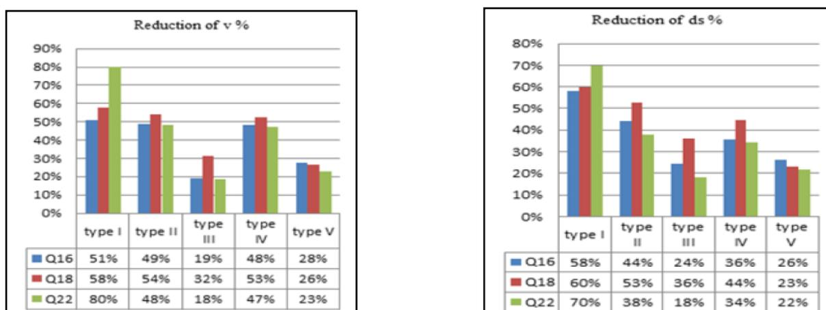
Figure.9 The diagram of reduction percent of maximum scour depth and volume given different types of piles positioning (Source: author)
