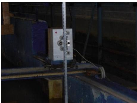
**Figure.3** The profile indicator to measure changes in bed depth (Source: author)
