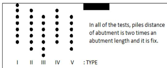
Figure.6 A view of locating abutment and piles (Source: author)
