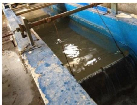
**Figure.2** The tail-water to adjust the downstream depth (Source: author)
