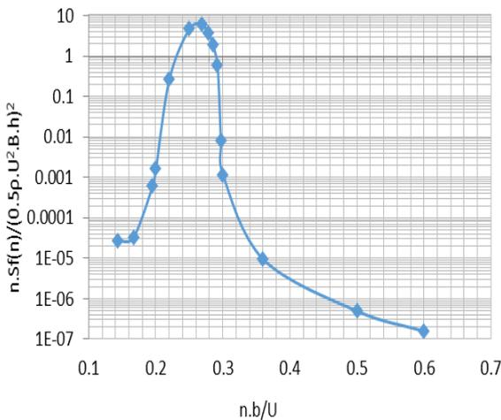
**Fig. 24.** The non-dimensional across-wind force spectrum when the length of plan is perpendicular with wind orientation (model a)
