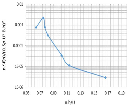
**Fig. 25.** The non-dimensional across-wind force spectrum when the width of plan is perpendicular with wind orientation (model b)
