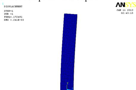
**Fig. 4.** Base mode shape in length of plan
