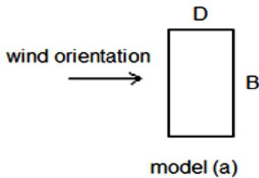
**Fig. 1.** length of plan is perpendicular with wind orientation (model a)
